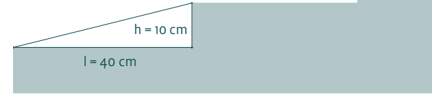
Abb. 2 Steigung = h : l = 10 \text{ cm} : 40 \text{ cm} = 0.25 = 25\%
